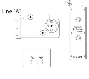
4. Drill a small hole using the pilot hole molded into the battery box top. Insert a medium size straight pin leaving the head approximately 2-3mm above the battery box top surface. The leather strap attaches to this fastener as the means for the battery box to be mounted to the wearers belt.
